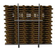
Put the double front-bar back in place and continue stacking panels on the other side.
